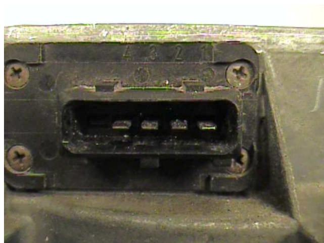
1. Push back the protection sleeve on the air flow sensor connector. The connector remains attached. Connect a voltmeter to terminals 9 and 6 on the back of the connector. Turn the ignition switch to the ON position. If you have an early 944 (pre-1985.5), the voltmeter will probably read approximately battery voltage (12 VDC). However, it should read a minimum of 8 VDC. If you have a late model 944, the voltmeter should read 5 VDC +/- 0.5. This is the AFM input voltage.
